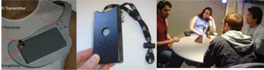
Figure 1: Different versions of the sociometric badge is shown in the left and in the middle. The sociometric badge is a wearable sensing device for collecting individual behavioral data. On the right is a group brainstorming session, and all participants were wearing the sociometric badges.
