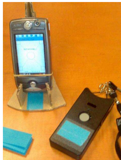
Figure 1. The Meeting Mediator: Sociometric badges (right bottom) capture group dynamics which is displayed as real-time feedback on mobile phones (left top).
