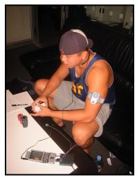
Figure 1: Subject wearing the non-invasive sensors (heart rate chest strap, finger skin conductance electrodes, audio microphone, and integrated motion/heat flux/skin conductance monitor along with the LiveNet platform running BioRecord during a session of the PokerMetrics Study. We use the collected physiology to correlate to manually recorded subjective outcomes such as stress level, interest, and bluffing.
