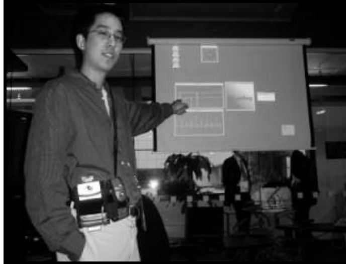
Figure 7: MIT.EDU application performing real-time FFT analysis and classification on accelerometer data, and wirelessly streaming real-time EKG/GSR/ temperature and classification results to a remote projector
