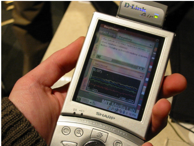
Figure 2: MIThril LiveNet wearable performing real-time FFT analysis and activity classification on accelerometer data, visualizing the results, as well as wirelessly streaming real-time EKG/GSR/temperature and classification results to a remote computer with a projection display as well as peer LiveNet systems that may be anywhere in the world.
