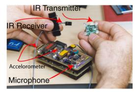
Figure 1 - The wearable sensor board
