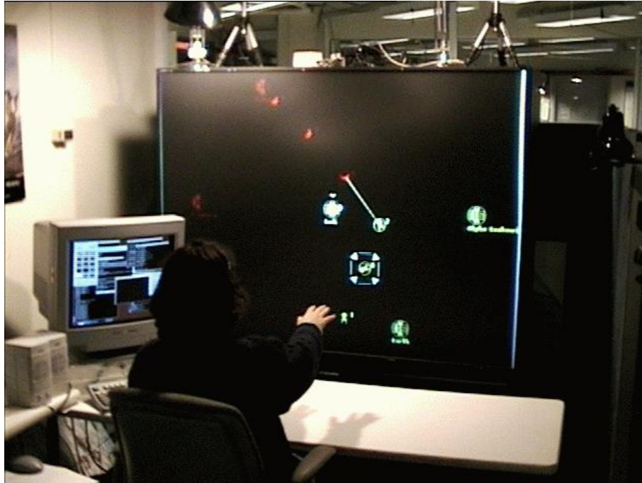
Figure 6-2: Netrek Collective Interface: the player uses a deictic gesture to select F0 . Cameras on top of the display track the player’s movements and a head-mounted microphone is used for speech recognition.
