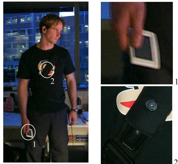
**Table 1** The labeling wearable: (1) the touch sensitive pad for Unistroke input, (2) sensor package containing pinhole CCD and boundary microphone.
