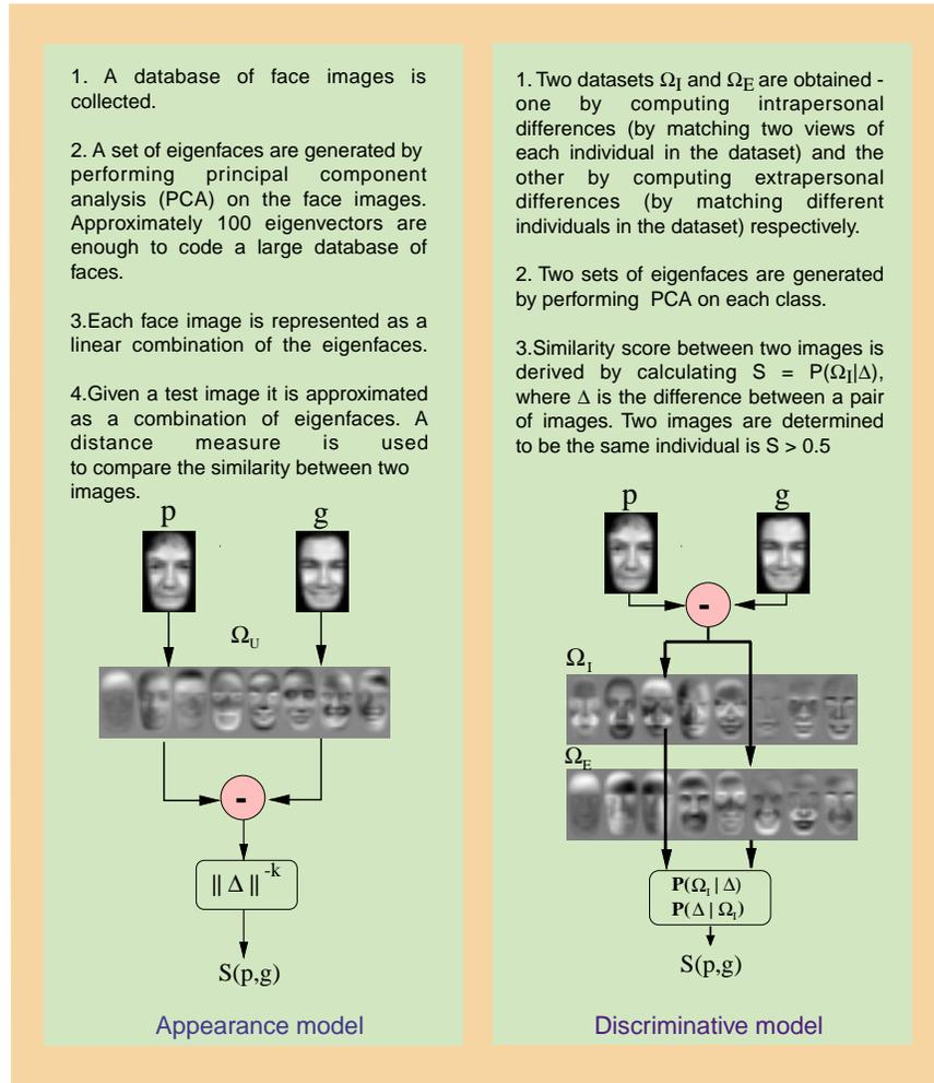
Figure 3: Face Recognition using Eigenfaces
