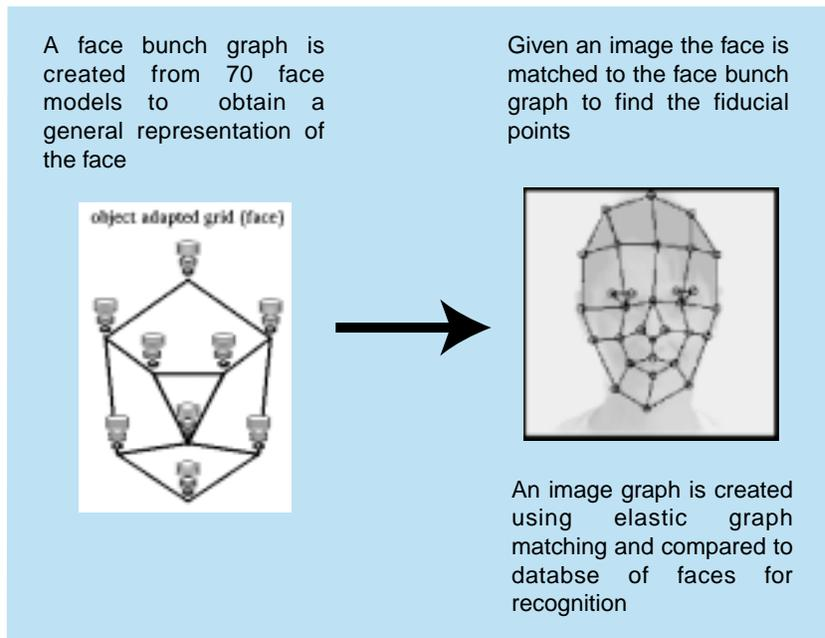
Figure 1: Face Recognition using Elastic Graph Matching
