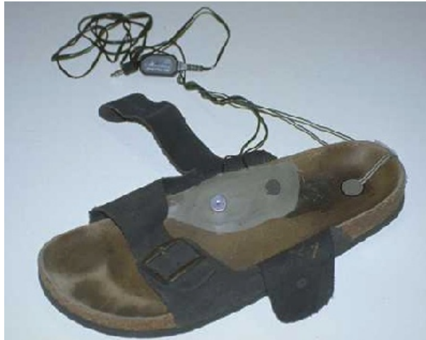
Figure 3: The shoe provides a convenient location for sensor placement. Here, a skin conductivity sensor is placed in the arch of the shoe and a pressure sensitive resistor is placed on the heel. Sensors look unobtrusive when worn. (Photograph courtesy of Fernando Padilla.)
