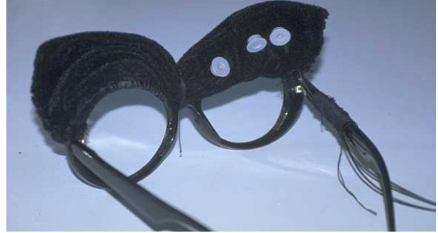
Figure 5: Glasses equipped with EMG sensors for detecting muscle movements used to recognize confusion. (Photograph courtesy of Fernando Padilla.)
