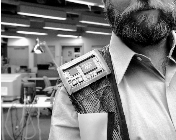
Figure 6: Embedded processor card integrated into Smart Vest and worn over a shirt.
