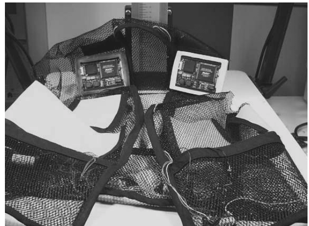
Figure 5: First Smart Vest constructed with twin processors, network connection and battery power.
