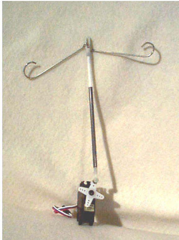
Figure 3-4: The Affective Tigger's ears are servo controlled. As the servo rotates down, it pulls on the push rod, causing the Affective Tigger's ears to go up.
