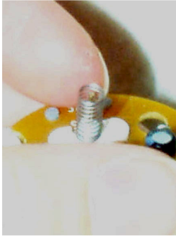
Figure 3-8: The abuse sensor is a simple post and coil accelerometer. A sharp blow or physical poke, as depicted here, will trigger the sensor.
