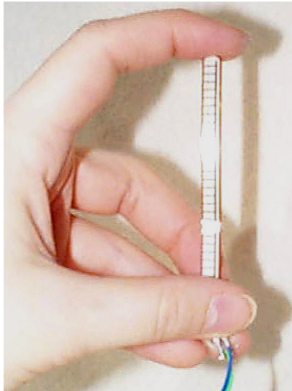
Figure 3-5: This is a commercially available resistor-type bend sensor. The strip only bends in one direction; the more it is bent the lower the resistance.
