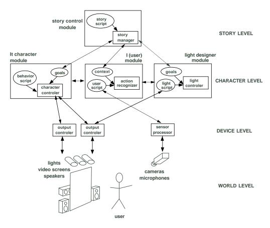
Figure 7.25 System architecture of "It".
