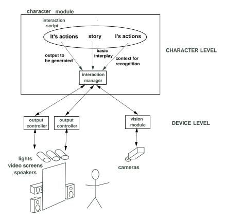
Figure 7.15 System architecture of "It / I".
