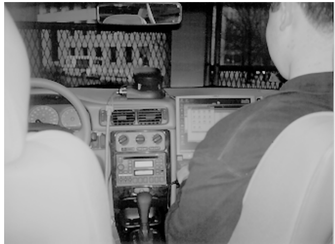
Figure 4: A camera placed on the front dashboard with a .42 wide angle lens captures context information from the road. An observer can note driving events and monitor sensors using a laptop.
