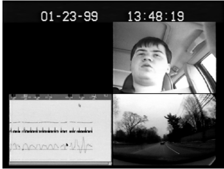
Figure 2: The four video inputs are displayed simultaneously. Shown are images from the camera mounted on the steering column (upper right), the dashboard (lower right) and the sensor system (lower left).
