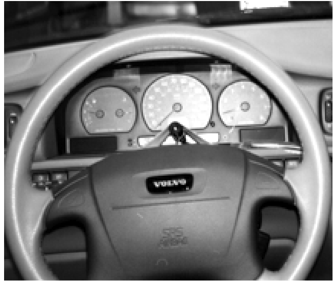
Figure 3: A small camera is placed on the steering column to capture facial expression while driving. The camera is placed behind the airbag release point to ensure the driver's safety.
