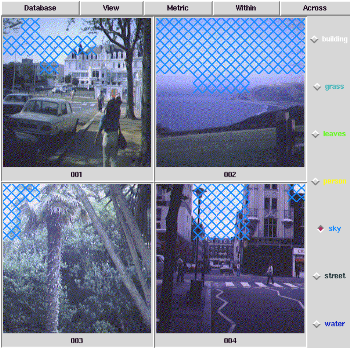
Figure 12: The FourEyes computer-assisted annotation tool. The user has mouse-clicked some patches of sky in the two right images, and assigned them the label “sky.” Within-image groupings allowed FourEyes to grow those labeled patches into larger “sky” regions (indicated by cross-hatching). Across-image groupings allowed FourEyes to also place tentative labels on the two left images. The menu buttons allow the user to control which sets of groupings are available to the learner.
