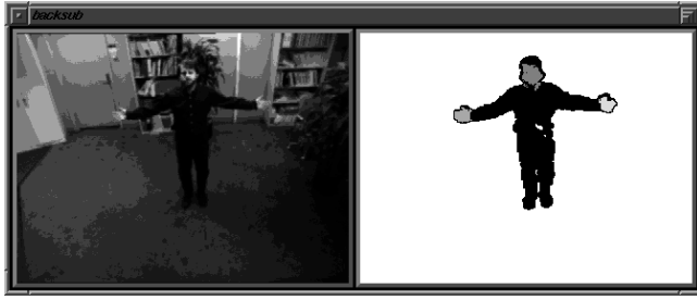
Figure 4: Backsub window showing a dithered sketch of the input video, figure/ground segmentation, and blob classifications (grey regions within the foreground silhouette).
