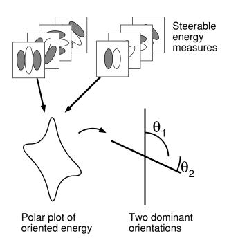
Figure 5-6: Initial processing in junction detection. A bank of steerable quadrature pair filters measures oriented energy as a function of angle. The two dominant orientations are defined to be the angles corresponding to the two strongest energy local maxima.
