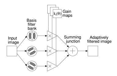
Figure 2-3: Steerable filter system block diagram. A bank of dedicated filters process the image. Their outputs are multiplied by a set of gain maps which adaptively control the orientation of the synthesized filter.
