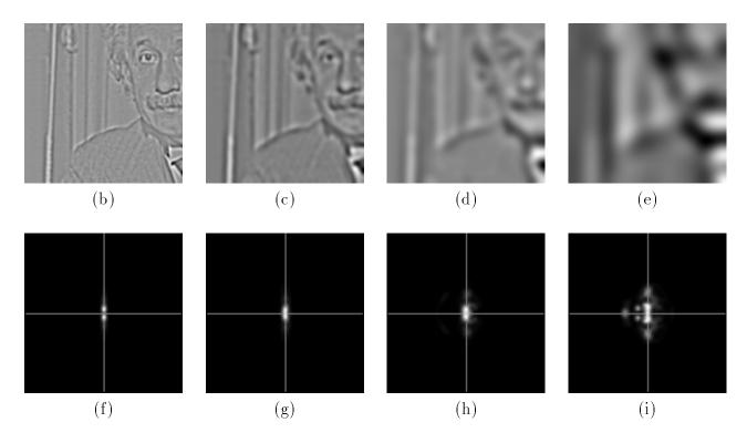
**Figure 4-4:** Effect of variation in scale on phase-energy histograms. (a) Test image, section of portrait of Einstein. (b) – (e) Test image bandpassed by four different scales of filters. (f) – (i) Corresponding phase-energy histograms. Notice that at scale (b), this image happens to be dominated by edge-phase contours, as seen in (f). At the coarser scales of analysis, many of the contours become of line or intermediate phase, as shown by the histograms (h) and (i).
