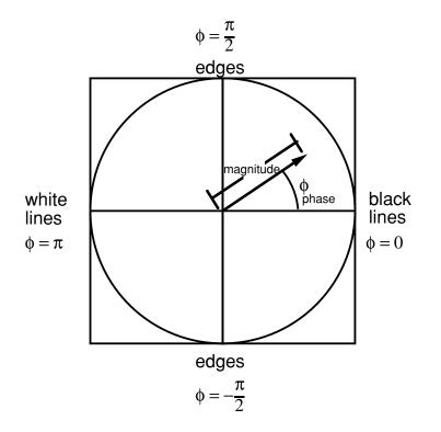
Figure 4-2: Explanation of phase-energy histogram intensities. In the image, a quadrature pair is steered along the locally dominant orientation of the image. From the quadrature pair outputs, magnitude and phase are measured positions of maximal energy response relative to displacements perpendicular to the dominant orientation. The intensity of the phase-energy histogram at a point is proportional to the number of measurements in the image at phase and peak magnitudes near that point.
