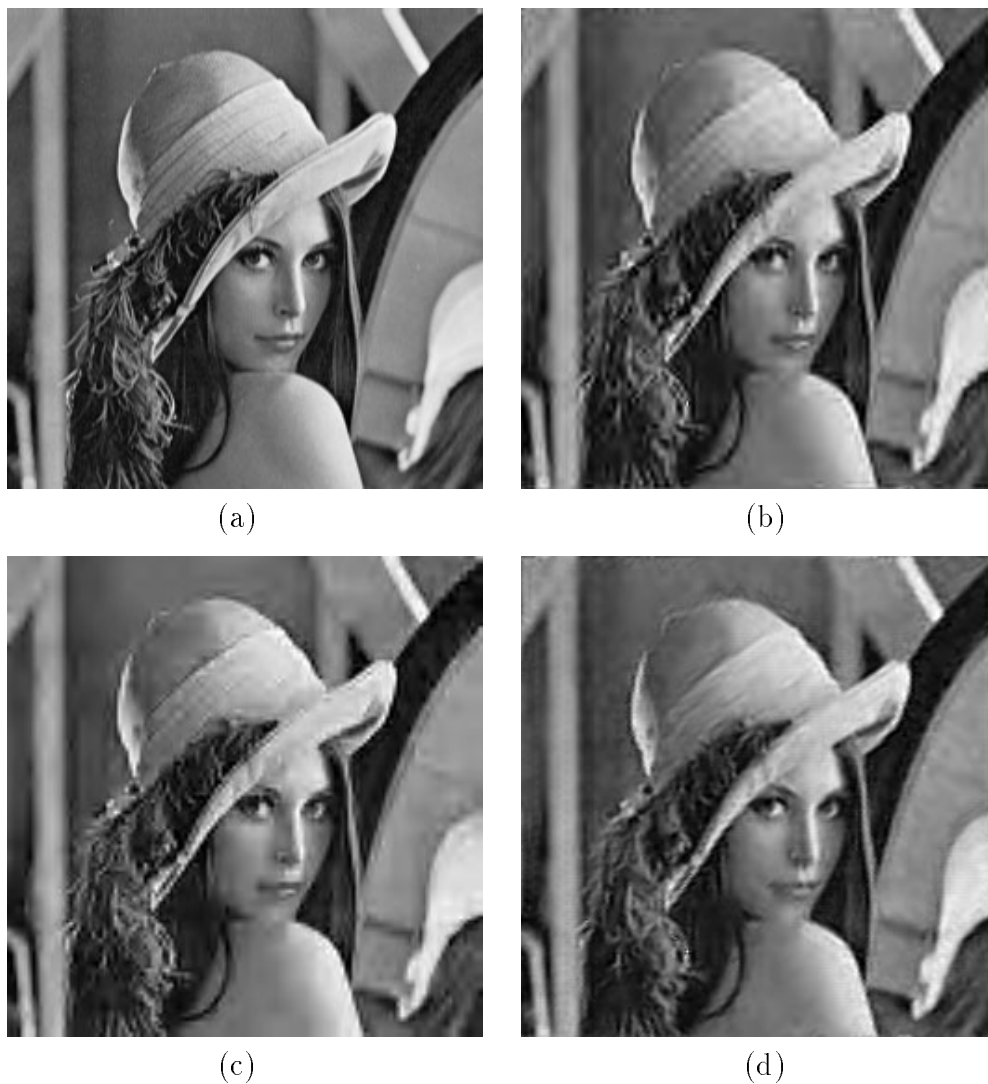
Figure 4.23: Data compression example using four-level pyramids. The pyramid data was compressed to a total of 16384 bits (i.e. total first-order entropy was 0.25 bit/pixel). (a) Original “Lena” image at 256 \times 256 pixels. (b) Compressed using 9-tap separable QMF bank. (c) Compressed using 3-tap asymmetrical filter bank. (d) Compressed using “4-ring” hexagonal QMF bank.
