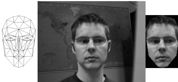
Figure 2: A generic 3D polygonal head model is aligned with a head-on shot of the video sequence, and the corresponding pixels are texture mapped to the surface of the face model.
